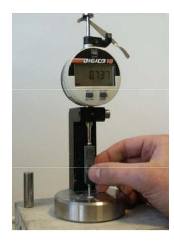
Mortar specimens 15x15x140mm with measuring studs at the ends
