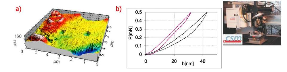
a) Effect of nanoindentation tests in the metal phase of sintered metal-ceramics composite (Mo+40%Al<sub>2</sub>O<sub>3</sub>).
